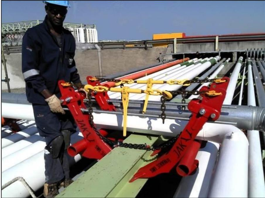
Lifts can be vertically secured by a double lock-out system on the jack, which is then declared a temporarily supported structure (no longer a suspended load) and therefore safe to work beneath.
